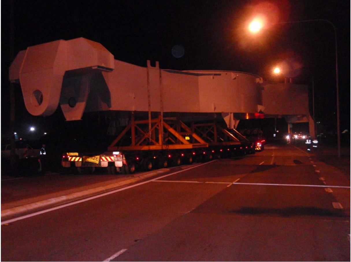
Figure 2.6: Stacker/Reclaimer Component Delivery
