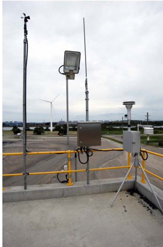
Figure 2.4: EBAM Dust Monitor installation
