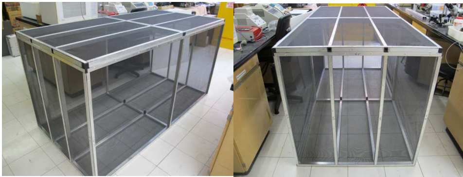
Figure 7. Basket (lateral and front view) to be used as experimental arena in the call attraction experiments. The basket is 2m long and can be fitted with solid dividers to form three chambers and run three replicates at once.
