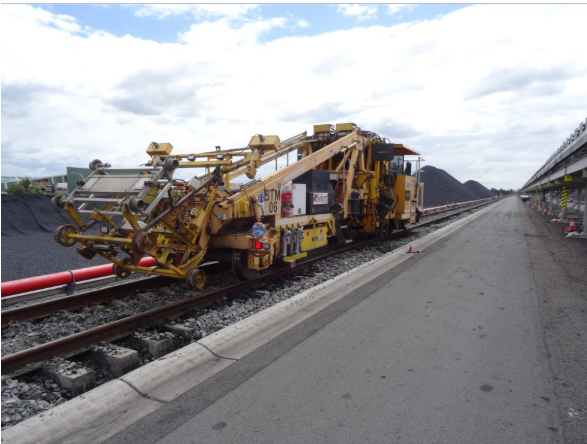
Figure 9: Tamping machine for stockyard rail maintenance
