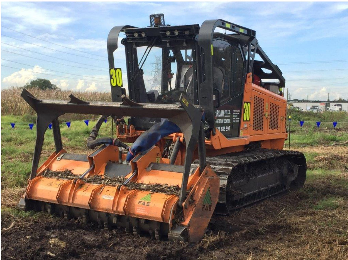
Plate 8: Mulcher used for mulching felled mangroves
